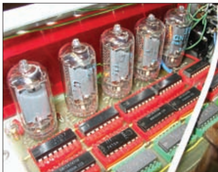
Fig. 4: This shows the rear view of the Nixies and their associated t.t.l. drivers in G3ZPF's d.f.m.
