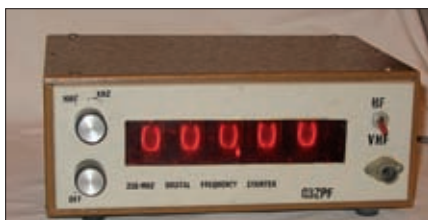
Fig. 3: This photograph David G3ZPF's d.f.m. which incorporated a mains power supply, even though it is very small for the time it was built.
