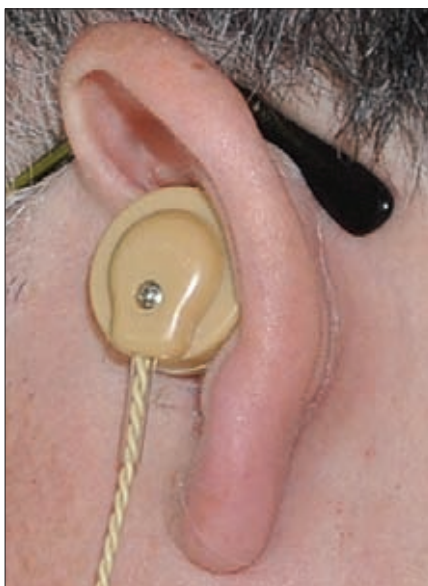
Fig. 6: A High impedance ear piece – ideal for use with simple crystal sets when good strength signals are available from the receiver .
