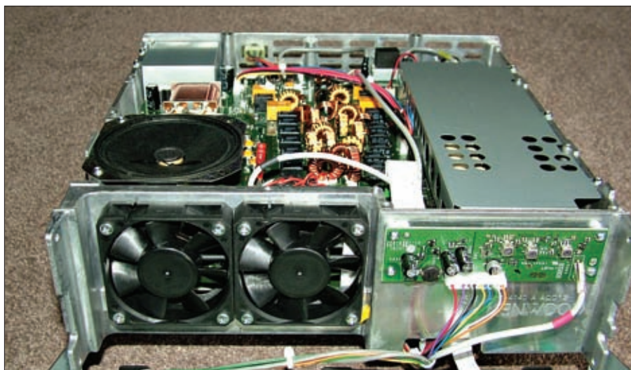
A pair of slow running 60mm square fans assist the cooling on the TS-590S.
