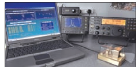
Paul EI5DI’s station showing WinKey , the Elecraft P3 and K3 and a single paddle key made by Scheunemann. The display on the P3 shows two c.w. signals spaced 300Hz apart. On a full screen scale of 2kHz it really makes a precision instrument Paul said!
