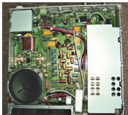
The main r.f. and filter board.
