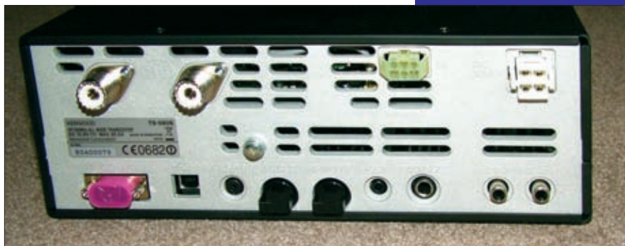
The rear panel of the transceiver showing the h.f. and 50MHz antenna inputs.
