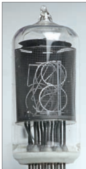
Fig. 5: The ten individual cathodes are shaped as numbers, the anode is the mesh in front of them all.
