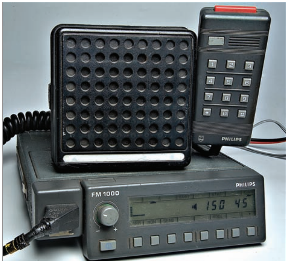
Fig. 2: A Philips FM1000 converted ex-PMR f.m. rig - a simple way of getting on 70MHz FM as mentioned in the text.
